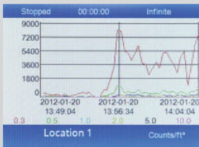
Profile of 0.3 to 10 µm particles captured over 15 minutes window.
